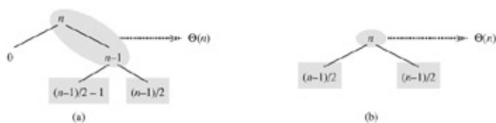
Figure 7.5: (a) Two levels of a recursion tree for quicksort. The partitioning at the root costs n and produces a "bad" split: two subarrays of sizes 0 and n - 1 . The partitioning of the subarray of size n - 1 costs n - 1 and produces a "good" split: subarrays of size (n - 1)/2 - 1 and (n -
