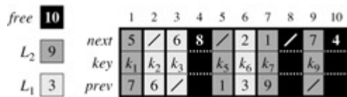
Figure 10.8: Two linked lists, L_1 (lightly shaded) and L_2 (heavily shaded), and a free list (darkened) intertwined.
